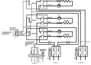
NOTE1: !:...! This symbol indicates the element is optional, The wiring type of the actual unit shall prevail. NOTE2:
