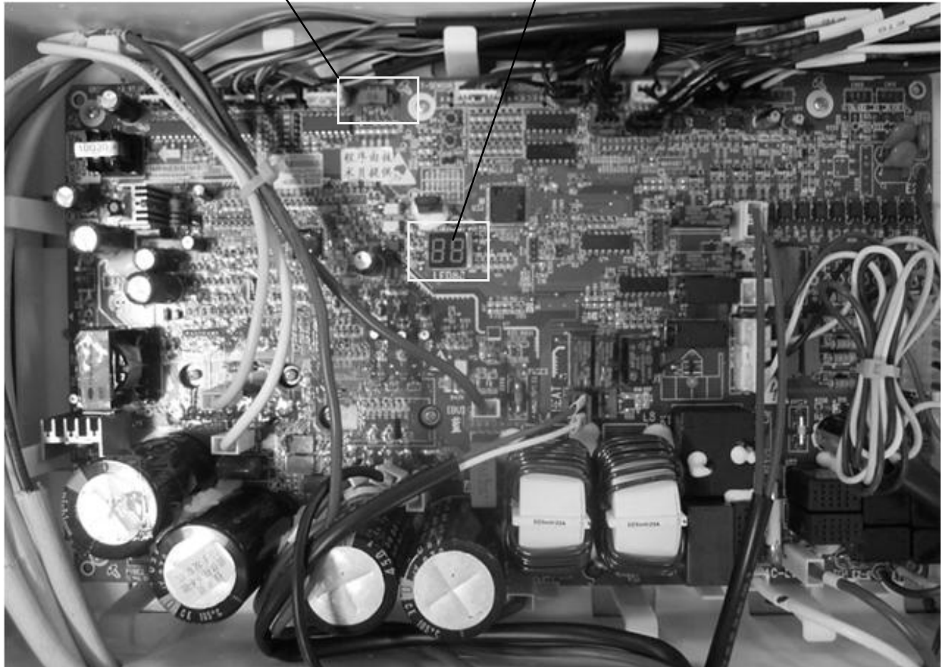
Main Board inside the control box.
