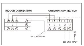
Wiring to the wired controller (7DP120XV included with the accessories.) See diagram below.
